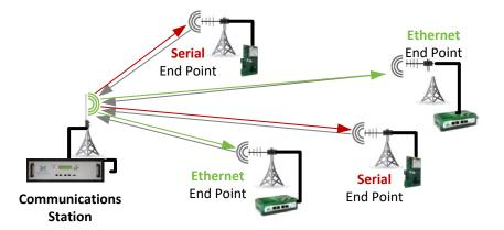
The XetaWave Communications Station continuously monitors remote serial and Ethernet end points and routers, both upstream and downstream, and provides a rapid, hot standby to ensure reliable, continuous network operation.
